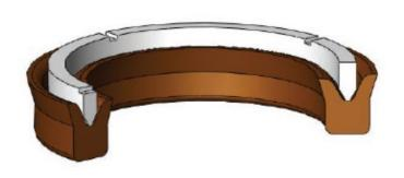
K153 is a two piece single acting low pressure chevron seal which consists of one special formulated reinforced cotton fabric with nitrile rubber sealing element and one thermoplastic header ring.
