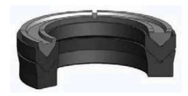
K03 is a three piece single acting sealing set which consists of one reinforced cotton fabric backup ring, one elastomeric nitrile rubber middle ring, and one thermoplastic header ring.
