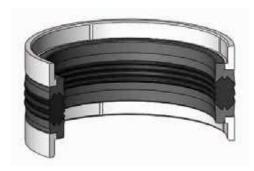
K42 is a five piece double acting compact seal which consists of one multiple lip elastomeric nitrile rubber sealing element, two polyester elastomer back-up rings on both sides to prevent extrusion into the sealing gap and two special profiled thermoplastic guide rings to absorb transverse forces.
