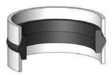
K20 is a three piece double acting compact seal which consists one elastomeric nitrile rubber sealing element and two special profil thermoplastic guide rings.
